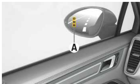
Fig. 89: Warning indicator A on door mirror
