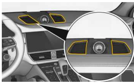
Fig. 22: Upper ventilation panel
