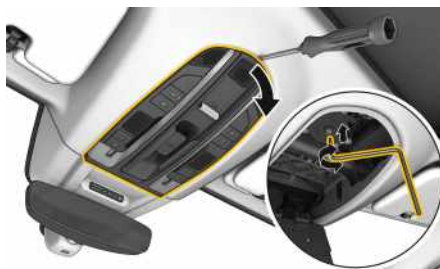
Fig. 165: Actuating roof system with the hexagon key
