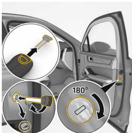
Fig. 43: Performing emergency locking of the passenger's door
