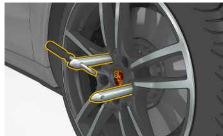
Fig. 234: Screw in two assembly aids on vehicles with PCCB
