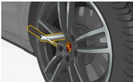
Fig. 233: Screw in one assembly aid on vehicles without PCCB
