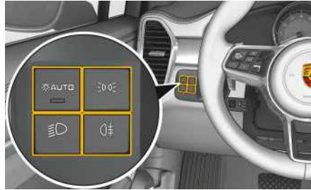
Fig. 99: Light control panel
