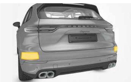
Fig. 90: Radar sensors in rear bumper
