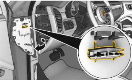
Fig. 70: Fuse box on the dashboard
