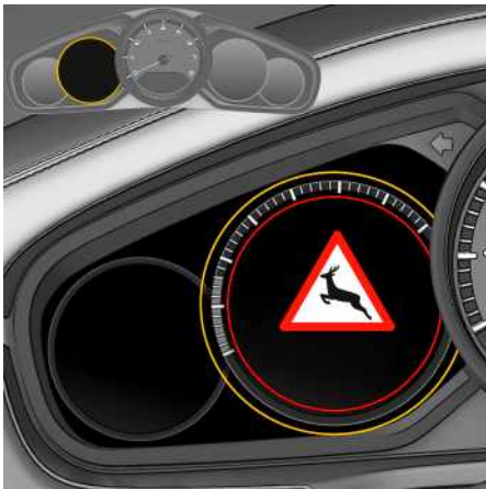
Fig. 124: Animal warning on the instrument cluster The animal warning reacts to hazards caused by large wild animals, e.g. deer, outside of built-up areas. The animal warning is triggered if an animal is in the projected driving lane or is dangerously close. The animal warning is deactivated automatically in urban areas in order to prevent it from being triggered by on-leash dogs for example.
