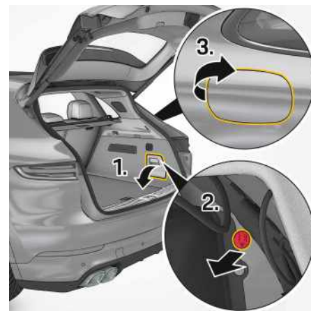
Fig. 159: Performing emergency release of filler flap
