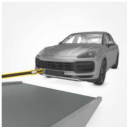
Fig. 209: Pulling vehicle onto flat bed
