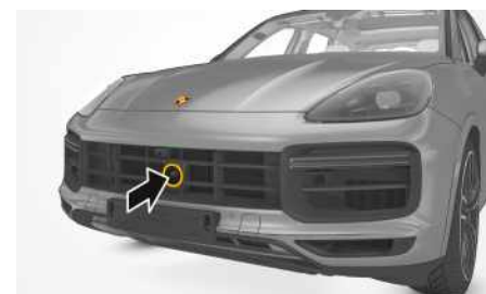
Fig. 10: Radar sensor position
