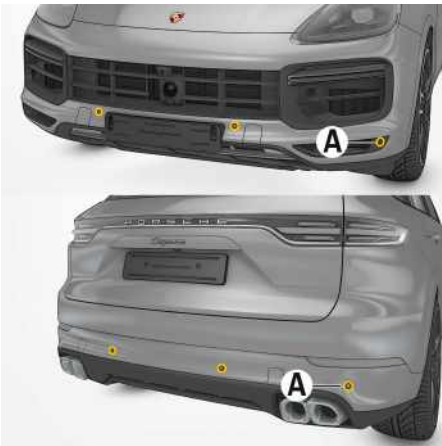
Fig. 129: Ultrasound sensors for distance measurement
