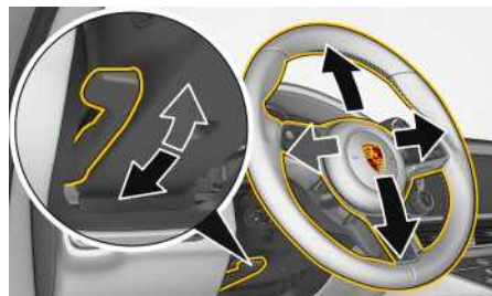
Fig. 195: Locking lever for manual steering wheel adjustment
