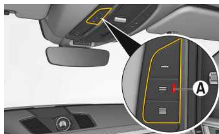
Fig. 74: Programming the garage door opener
