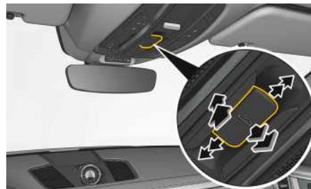
Fig. 162: Opening and closing the roof system
