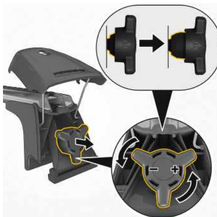
Fig. 169: Remove the fastening screw and turn counter-clockwise.
