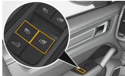
Fig. 237: Power window/sunblind switch on driver's door
