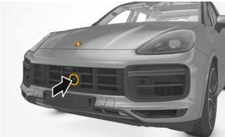
Fig. 3: Radar sensor position
