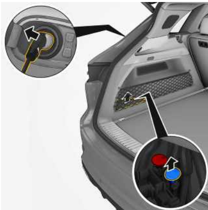
Fig. 51: Performing emergency release of the vehicle plug (vehicles without DVD changer)
