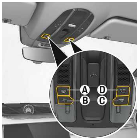
Fig. 81: Operating interior lighting
