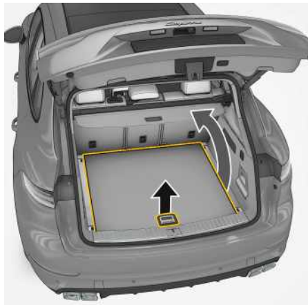
Fig. 103: Opening the cargo area floor
