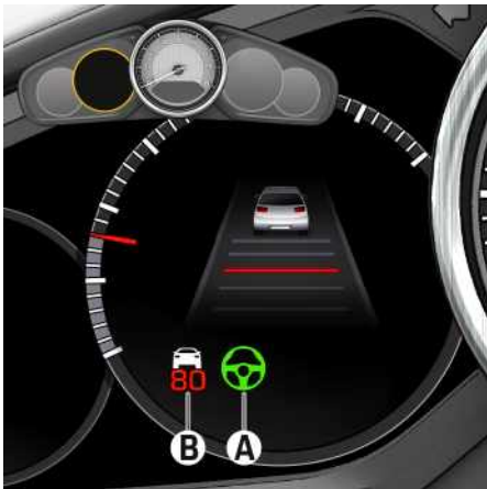
Fig. 2: Active Line Keeping in the Speed & Assist display A Active Line Keeping status display B The ACC status display with desired speed and vehicle ahead
